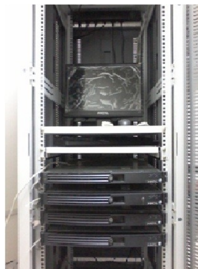
Workstation useful for Molecular Docking, QSAR, Pathways Modeling and Simulation High Performance Cluster with One master node and three slave useful for Molecular Dynamics
